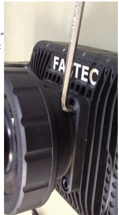
Figure 7-11: Removing an F- or PL-mount
